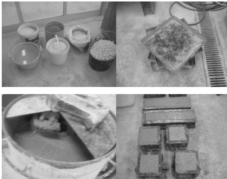
Figure 6: Concrete mixing & sample preparation
