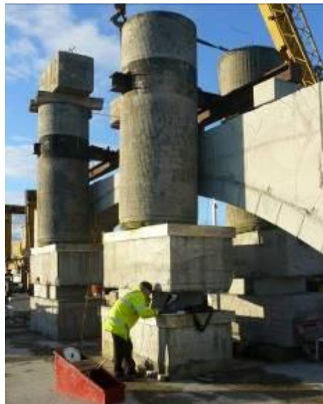
Figure 3 Testing full scale 15m span 'FlexiArch'
