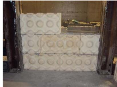
**Fig. 7** Construction of specimen to uniaxial compression tests on high size specimens
