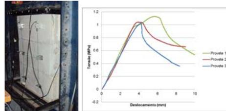
**Fig. 7** Results of the experimental tests; (a) force-displacement diagrams; (b) cracking pattern
