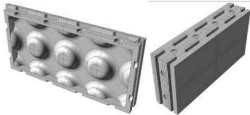
**Fig. 1** Shape of the composite block for partition walls
