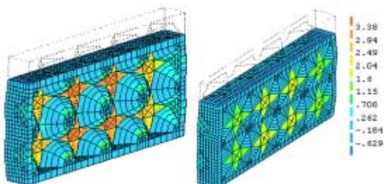
**Fig. 5** Numerical simulation of composite blocks under compression
